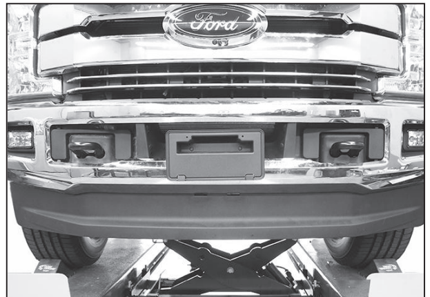
(Fig 6) Remove plastic air dam from bumper
