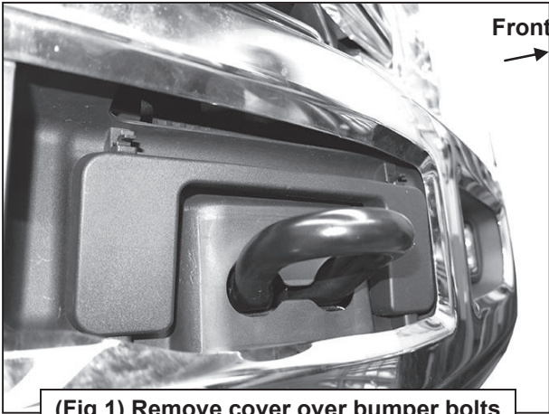
(Fig 1) Remove cover over bumper bolts
