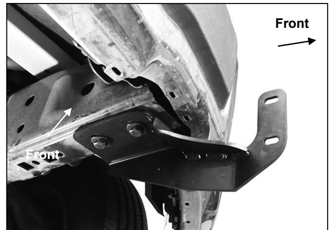
(Fig 16) Attach Frame Bracket to Nut Plate.
