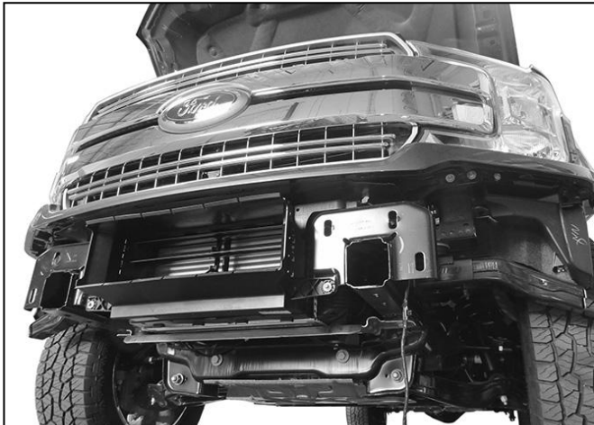
(Fig 18) 2018 models: Remove bumper assembly
