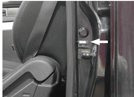
Front Center of sensor 1" down from center of door bumper circle
