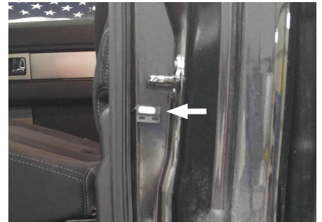
Rear Center of sensor 1-1/4" down from door latch
