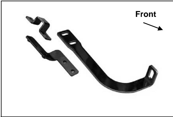
(Fig 13) Driver side Top Brackets pictured
