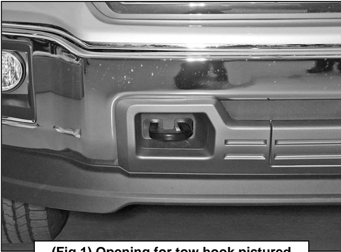
(Fig 1) Opening for tow hook pictured
