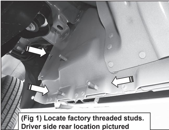
**(Fig 1) Locate factory threaded studs. Driver side rear location pictured**
