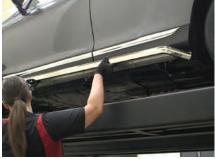
Attach the running board to the brackets using six 8mm bolts, six 8mm nuts, six 8mm lock washers and six 8mm flat washers.
