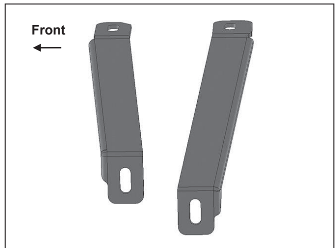
(Fig 6) Driver/left Front and Rear Support Brackets. NOTE: Front Support Bracket (left) is shorter than the rear (right).
