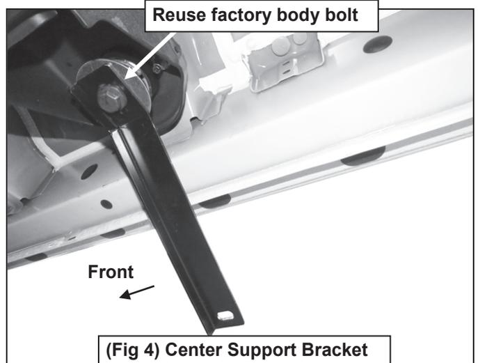
(Fig 4) Center Support Bracket attached to center body mount
