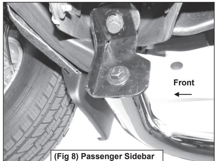
(Fig 8) Passenger Sidebar attached to Front Bracket
