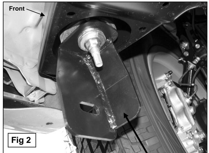
Install the front Mounting Bracket with the gusset toward the front of the vehicle.
