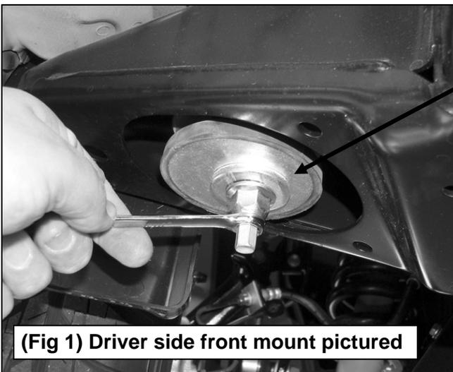
To prevent the factory center bolt from spinning, hold the center bolt with a wrench as you loosen or tighten the factory hex nut. Do not remove the center bolt or the rubber body mount.
