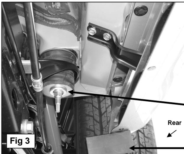
Remove factory hex nut and washer. See Fig 1 for information. Driver side rear body mount pictured.
