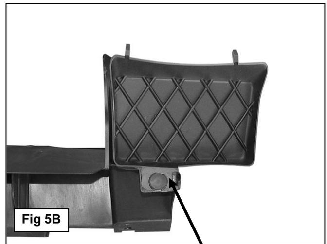
Remove (2) factory clips to remove the block off cover from each end of the air deflector. 2011-13 driver side of air deflector pictured
