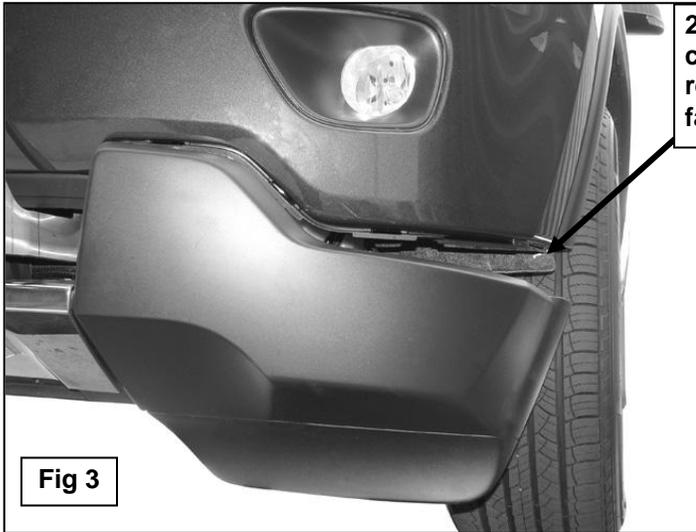
2011-13 vehicles: Remove factory hardware and release clips at ends of lower bumper cover only. Do not remove lower bumper cover. (For vehicles without factory tow hooks only)
