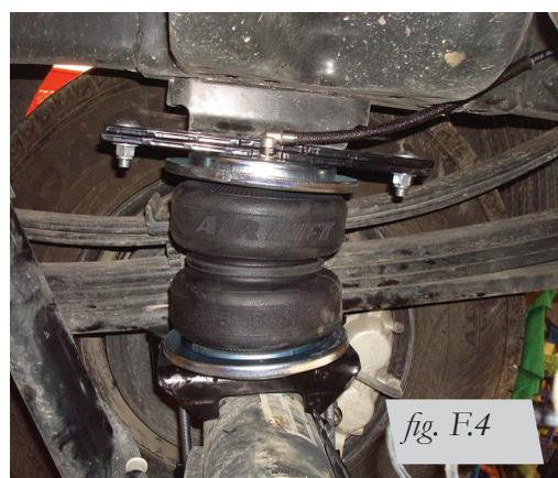
Inside view of the passenger's side installation.
