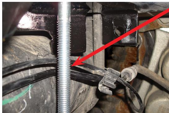
The carriage bolt is always on the outside of the brake line on the passenger's side, regardless of the year.
