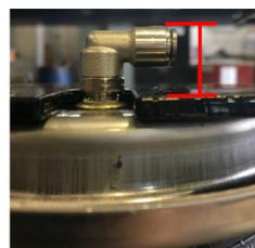
Ensure fitting is less than 7/8" in height
