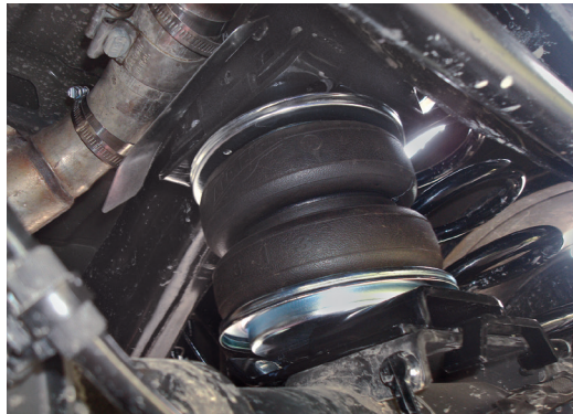
fig. F.3 Inside, rear of axle view of passenger's (right) side installation.
