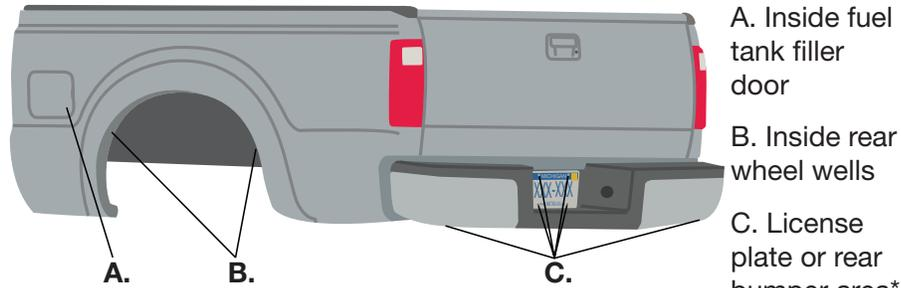
\* For LoadLifter Ultimate Plus kits, the recommended location for the Schrader valves is the rear bumper area or license plate.
