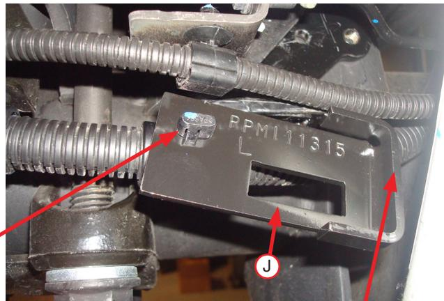
**Insert tab on ABS wire loom here**
