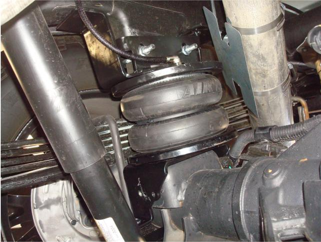
Inside, forward of axle view of driver's (left) side installation.
