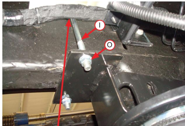
**Do not pinch the wiring harness when installing the U-bolt**
