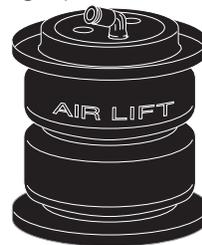
2. Install the air fitting (E) finger tight plus 1 and 1/2 turns (Fig. 4). Use a 7/16" open end wrench, being careful to tighten on the metal hex nut only. *Do not overtighten.* This fitting is precoated with sealant.
