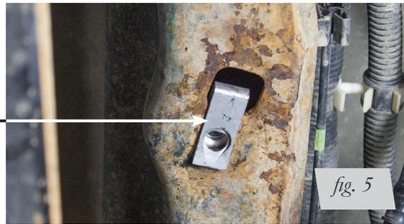
5. All years: On the right side (passenger's side) there is an emergency brake cable holder that is bolted on to a bracket welded to the axle, with a self-taping bolt. In order to make clearance for the axle strap, it will be necessary to cut this off and/or grind this bolt flush to the bracket (Fig. 6).
