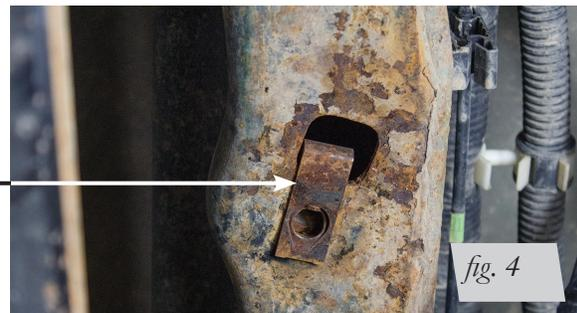
4. For the early 04-08 models, install a new Universal Nut (V) into the large hole so that the threaded portion is up inside the frame (Fig. 5).
