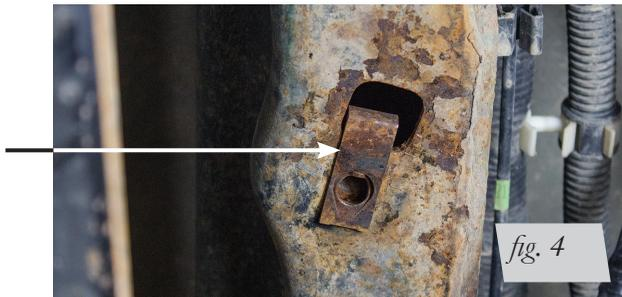
4. For the early 2004-08 models, install a new universal nut (M) into the large hole so that the threaded portion is up inside the frame (Fig. 5).
