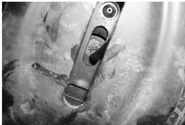
Bottom view showing air line inside of A-arm
