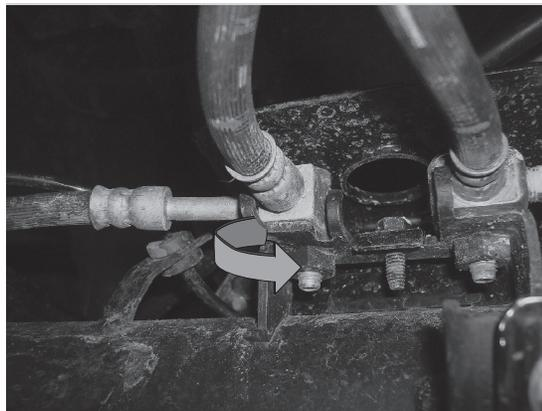
Loosen the bolt holding the brake line to the axle bracket and rotate the brake line counterclockwise as far as it can go. Tighten the brake line bolt so the line stays in this position.
