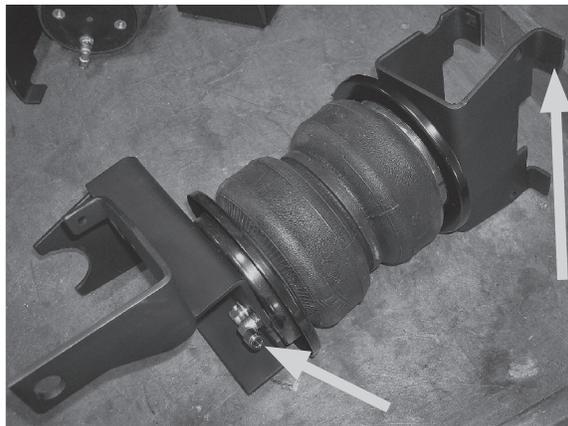
The flanges on the lower brackets must face the same direction as the fittings on the upper assemblies.
