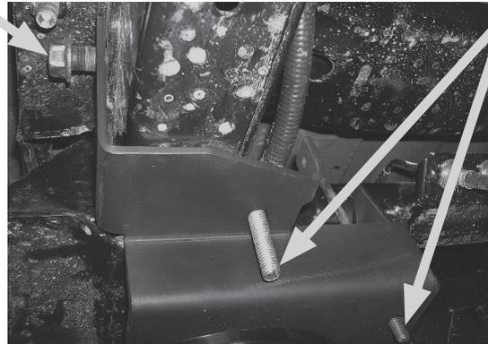
While raising the axle, once the assemblies are in place, align the J-bolt and round U-bolt with the corresponding holes in the upper brackets.
