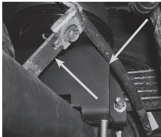
Bend the bracket slightly to gain clearance between the emergency brake line and lower bracket forward of the axle on both sides.
