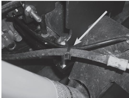
Tie strap the ABS line to the brake line as shown on the driver's (left) side
