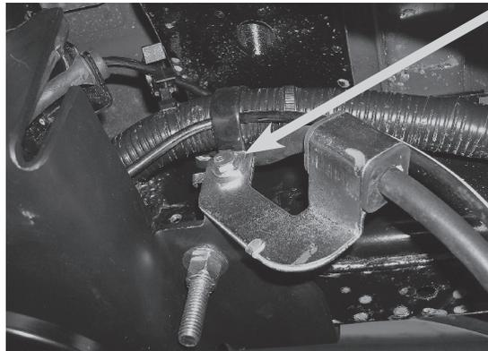
Reattach the previously removed ABS line and axle vent tube bracket on the passenger's (right) side using a P-clamp.
