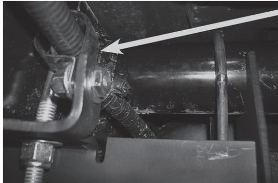
Reattach previously removed wiring onto the upper bracket on the driver's (left) side.
