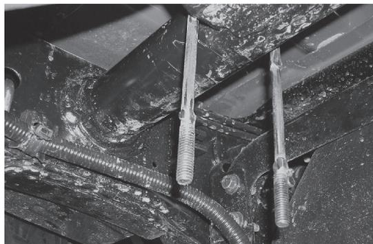
Set the round U-bolts around the cross member over the axle, as shown, on both driver's (left) and passenger's (right) sides. Be careful not to pinch any wiring that may be in the area on the driver's (left) side.
