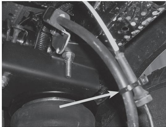
Tie strap the ABS line to the axle vent tube, as shown on the passenger's (right) side.
