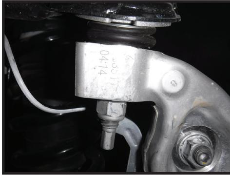
5. Separate the UCA from the spindle and support the spindle so that it does not overextend the CV joints when detached.
