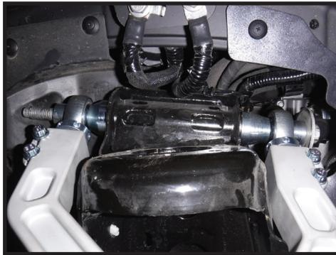
8. Pivot the Delta Joint stem so that it is inline with the taper bore in the spindle. The new Delta Joint will be very stiff the first time you move it. Rotate the upper control arm downward and install the stem through the spindle taper. Install two washers per side with the supplied flanged nut on the taper pin. Connect the UCA to the spindle using an 18mm. [Torque to 60 ft-lbs]
