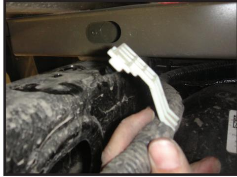
**5.** Move the exhaust on the passenger side of the vehicle. Loosen the exhaust clamps forward of the muffler. Remove the exhaust hangers just rear of the axle on both sides. Remove the two bolts from the rear exhaust hanger where it attaches to the bumper on each side, set aside for reinstallation later. The exhaust can now drop down out of the way to allow for bracket installation. A bungee or strap can be used to help support some of the weight in the lowered position. [FIGURE 5 - 8]
