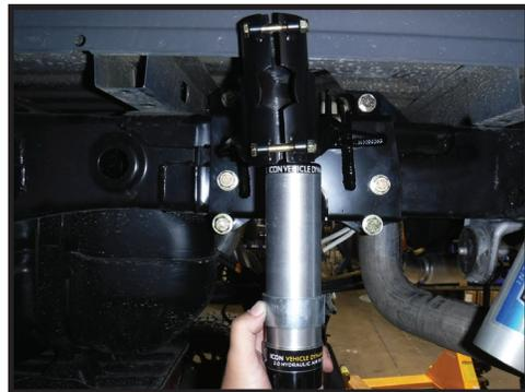
**21.** Install the striker pads on the axle tube. Pop the ABS clip from the tab on the axle tube. The lower portion of the striker plate hooks under the leaf spring pad on the axle. The slot where the ABS tab was will need to be opened up for the bolt that will secure the striker. Standard drill bits will tend to catch in the oval hole, a die grinder is recommended. Tighten until the pad is in full contact with the axle tube but do not overtighten. [FIGURE 30 - 33]
