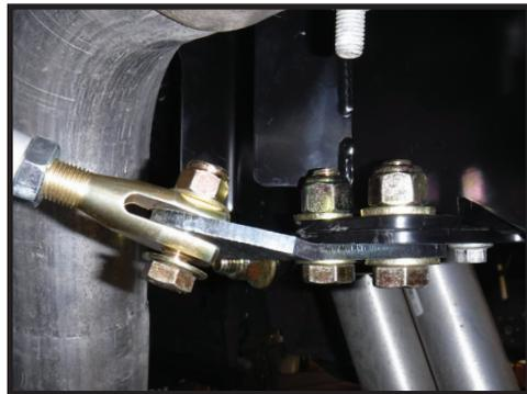
**17.** The crossmember is in slotted holes. Center it left to right and tighten the (4) bolts to 78 ft-lbs.
