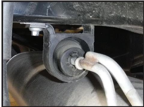
**6.** To clear the crossmember the exhaust will need to be positioned rearward. This is done by sliding the rear half of the exhaust out of the slip joint at the clamps by 3/4". [FIGURE 9 & 10]
