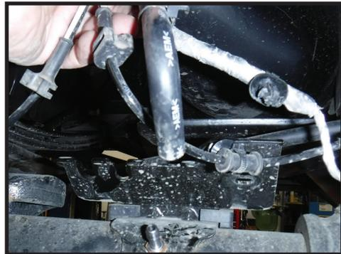
**23.** Install the low profile ABS and vent line bracket. Remove the ABS and grommets from there slots, wire clips and vent hose. Unscrew the vent fitting from the axle and remove bracket. Install the low profile bracket with the factory vent fitting. Again, you will need to reposition the grommets on the ABS wires. Slide until they can be reinserted in the bracket and make sure there is adequate slack in all parts of the wires. Reinstall the vent hose on the fitting. [FIGURE 36 & 37]
