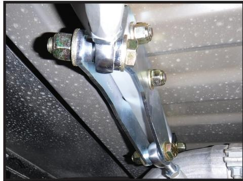
**16.** Install the tension rod strut tabs on each side. IMPORTANT: on the driver side the tab goes ABOVE the tabs on the inner and outer bracket and on the passenger side it goes BELOW the tabs on the inner and outer bracket. Secure with (2) 1/2" x 1.25" bolts, washers, and nuts on each side. [FIGURE 26 & 27]
