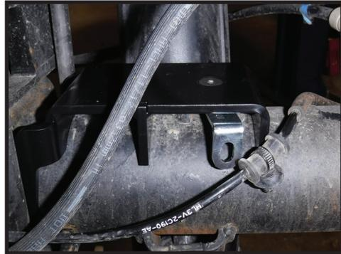
**22.** Install ABS clip in the striker nut plate. The clips will need to be repositioned to allow slack in the ABS wire. Slide the rubber grommets in the clip and the next closest clip under the leaf spring, use lube or soapy water to ease sliding them. [FIGURE 34 & 35]
