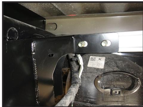
**13.** As you slide the outer brackets into position on the frame, make sure the nut plate is located correctly inside the frame with its locating washer on the rearward hole. You can snug up the fully threaded bolts to make sure it stays in place but do not tighten them. [FIGURE 21 & 22]
