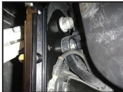
**7.** Install the ICON coilover assembly. Install the heim spacers in the lower control arm with the shorter one towards the front of the truck. Make sure the spacers in the lower eyelet of the shock are oriented correctly. It helps to get the 3/8" x 1" upper bolts ready with the lock washers on them and placed in a easy to reach spot once you get the coilover up in position, as the coilover assembly is very heavy, an extra set of hands is recommended for this step.
