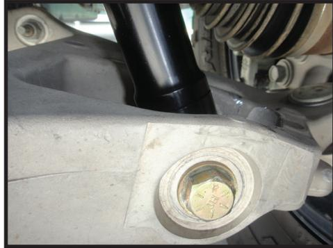
**9.** Install the lower 5/8" x 5" bolt and washer through the lower pivot then install the second washer and nut. [Torque to 120 ft-lbs]
