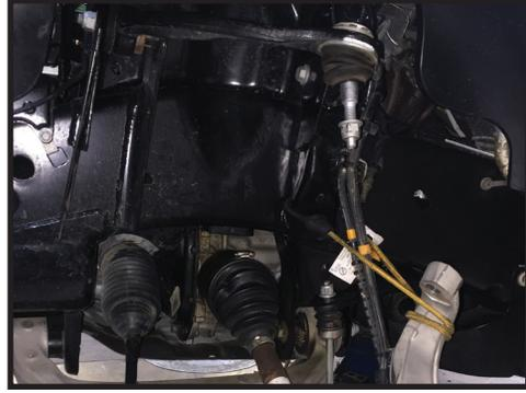
**4.** Remove the lower shock bolt (30mm nut, 27mm head). Remove the (3) upper shock mount bolts. NOTE: Do not loosen the center nut on the top of the shock or the assembly can come apart violently, resulting in damage and serious injury. Remove the shock assembly from the vehicle. You will have to push down on the lower control arm to get the bottom of the shock to come out of its pocket in the arm. If the knuckle is held slightly outward from vertical then the arm will extend downward easier.
