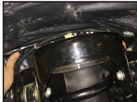
**3.** Disconnect the tie rod and upper control arm from the knuckle. Loosen the nuts (18mm and 21mm) and strike the side of the knuckle at the taper to dislodge. Tie or bungee cord the top of the knuckle to prevent it from flopping outward and overextending the CV joints. Disconnect the sway bar link at the sway bar using an 18mm. [FIGURE 3 & 4]
