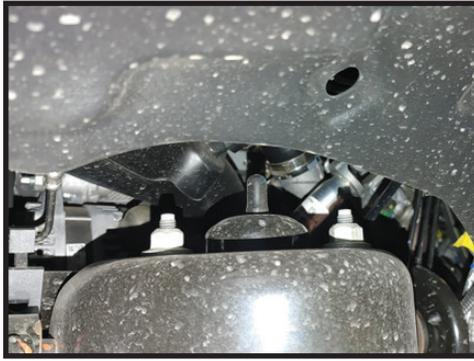
**7.** If the lower arm was removed, Reinstall it now, only snugging the bolts in place (They will be torqued at the end).
