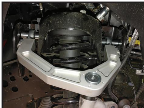
20. Tighten the UCA bolts at the chassis using a 21mm and 18mm socket/wrench. [Torque to factory spec]
