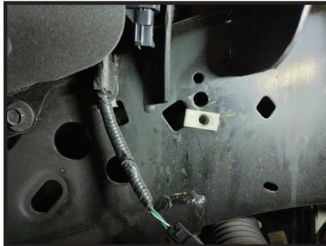
**16.** Install the bracket and sensor tab into the old bolt hole and use the factory hardware to secure it into the new location.
