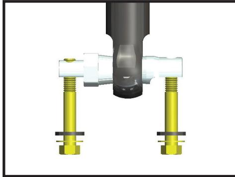
**11.** Connect the upper control arm to the spindle using an 18mm socket/wrench. [Torque OEM balljoint to factory spec] [75 ft-lbs for the ICON DELTA JOINT]
