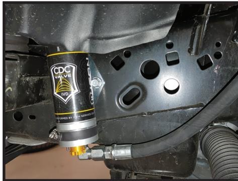
**15.** Mount the reservoir to the bracket using supplied hose clamps and a flat head screw driver or 5/16" socket/wrench.
