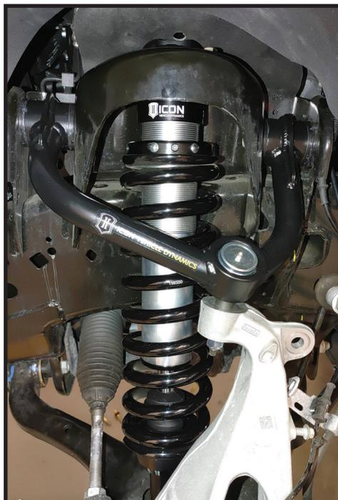
**10.** Use the supplied 7/16" bolts and washers to secure the ICON coil-over to the lower arm using a 5/8" wrench/socket [Torque to 50 ft-lbs]. Each 7/16" bolt will get 2 washers, the thicker black oxide washer will go against the Lower control arm, while the thinner yellow zinc washer will go against the head of the bolt. [FIGURE 6]
