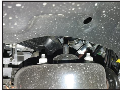
**7.** If the Lower arm was removed, re-install it at this time. Do not torque the pivot bolts until the truck is sitting on its own weight.
