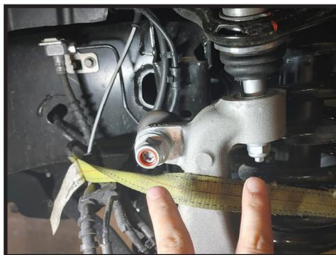
**10.** Remove the UCA from the frame using a 21mm and 18mm socket/wrench.
