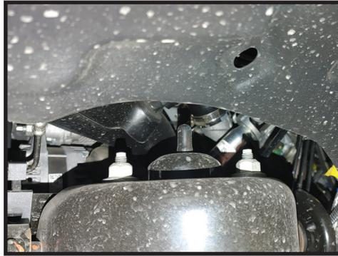
**7.** If the lower arm was removed, Reinstall it now, only snugging the bolts in place. [They will be torqued at the end]
