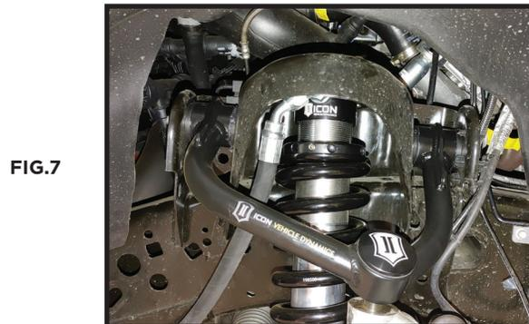
**17.** Tighten the UCA bolts at the chassis using a 21mm and 18mm socket/wrench. [Torque to factory spec]
