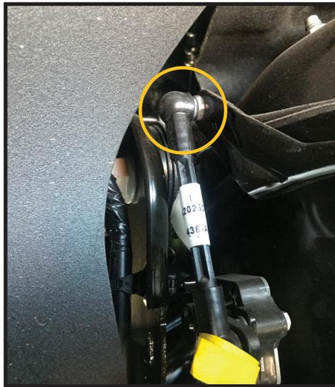
**9.** Remove the sway-bar link and upper control arm from the spindle. Support spindle with a jack or strap to prevent the CV (4x4) or brake lines from over extending. (18mm, 21mm, T45 Torx) [FIGURE 4]
