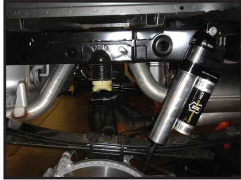
**6.** Remove the factory parking brake cable bracket from the differential using a 10mm socket/wrench. Pry the bracket opened, and remove it from the cable. [FIGURE 6]
