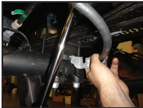
**7.** Slide the supplied parking brake cable bracket over the metal sleeve on the cable. Connect it to the differential using the factory screw and a 10mm socket/wrench. [Torque to factory spec] [FIGURE 7]
