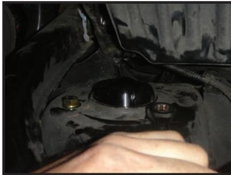
**10.** Reconnect the sway bar links to the sway bar using a 17mm. [Torque to factory spec]
