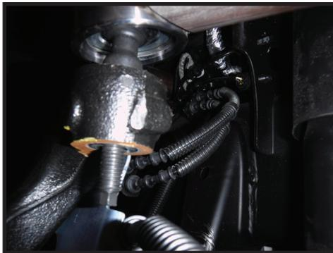
**13.** Before tightening the factory hardware, grease the pivots at the zerk fittings with a grease gun until grease begins to come out of the bushing housing.
