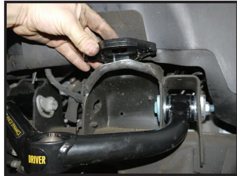
**23.** Slide the shock into the shock mount making sure to have the bushings on prior to final installation.
