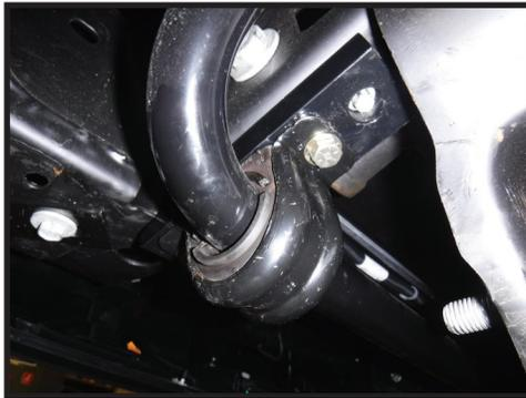
6. Using a jack, slightly lift the lower control arm to prevent the suspension from being at full droop.
