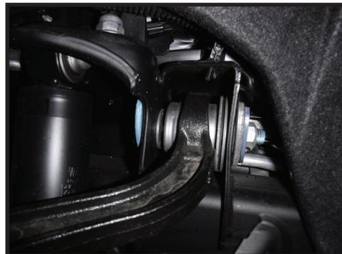
**10.** Before installing your new upper control arms, care must be taken to grease the bushings (liberally) prior to installing assembly. Failure to grease properly will cause premature bushing wear and increased noise.
