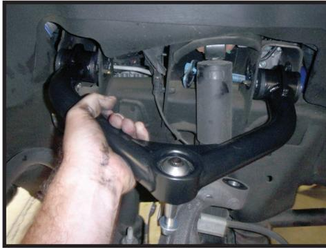
**12.** Line up the taper pin with the spindle and insert it without damaging the threads. Use supplied flanged nut to install the taper to the spindle. [Torque to 60 ft-lbs] [FIGURE 8]
