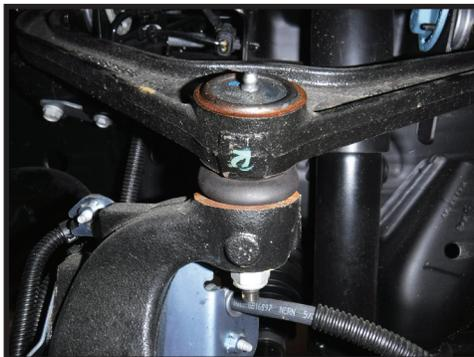
8. The spindle will need to be supported so that it will not overextend the CV's on 4wd models, or possibly damage steering components. Using a ball joint separator, detach the ball joint from spindle.
