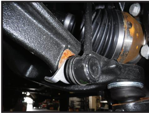
4. Using the factory bolts, connect the sway bar relocation bracket to the frame. Torque to factory spec using a 10mm.
