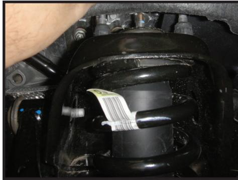
**7.** Remove lower bolt using a 21mm socket/wrench.
