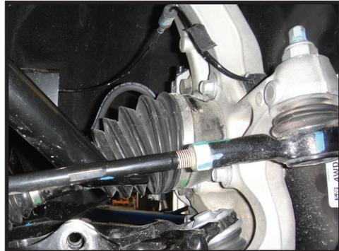
**20.** Reconnect the tie rod to the knuckle using a 21mm socket/wrench. [Torque to factory spec] (FIGURE 20)
