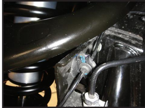
**18.** Verify that brake line tab, UCA and reservoir hose do not make contact at full droop. Failure to route the hose properly can cause damage to the hose which is NOT covered under warranty. (FIGURE 18)
