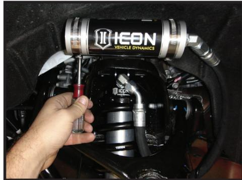
**14.** Mount the reservoir to the reservoir mount using the supplied hose clamps and a 5/16" nut driver. (FIGURE 13)
