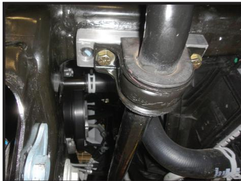
**16.** Using a 13mm socket/wrench loosen the brake line bracket on the coil bucket. Push it down and slightly bend it rearward. [Torque to factory spec] (FIGURE 15 & 16)
