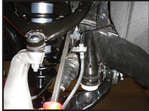
**17.** Reattach the UCA to the knuckle using a 18mm socket/wrench. [Torque to factory spec] (FIGURE 17)
