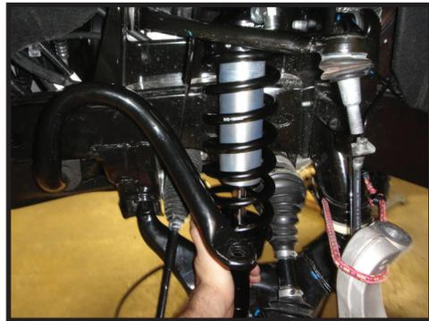
**10.** With the OEM coilover removed, sway bar removed, and UCA free from the knuckle, sand the lower shock tab as shown. Failure to sand this section will allow the CV boot to rub at full droop and full steering lock. Be careful not to hit the CV boot. (FIGURE 7 & 8)
