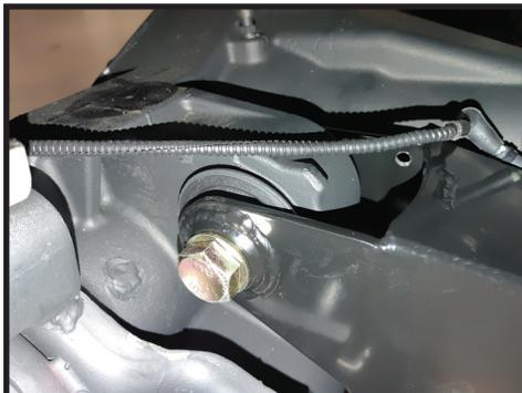
9. Install the radius arm into the frame pocket and use the OEM bolt and nut. [FIGURE 7]
