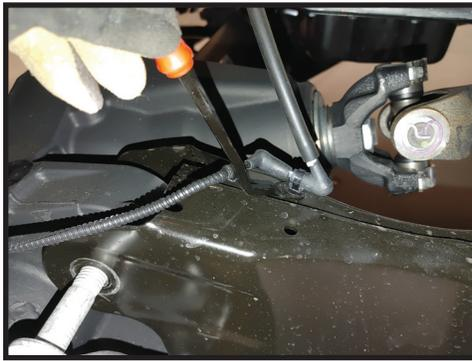
**4.** Support the radius arm and remove the frame side bolt using a 24 and 27mm wrench/socket. [FIGURE 4]
