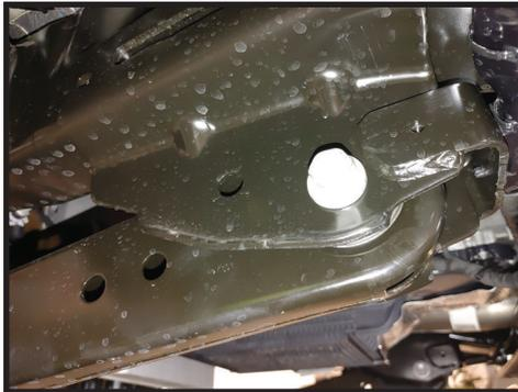
**5.** Remove the 2 bolts on the axle mounts using a 24mm. Remove the radius arm.
