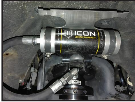
**12.** If installing coilover conversion, use the doubler reservoir mount (supplied in coilover kit) for mounting both reservoirs as shown. **[FIGURE 5]**
