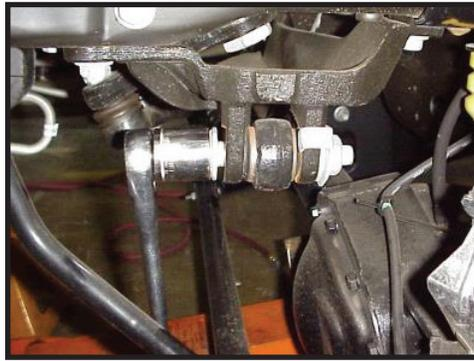
5. Use a jack to support the axle and then remove the factory shock using a 17mm and 18mm socket/wrench.
