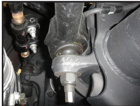
4. Loosen the pinch bolts using a 3/8" 12pt socket/wrench.
