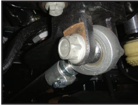
**NOTE:** This track bar is adjustable from 36.75" - 37.75". The stock track bar measures 36.625" from eye to eye.
