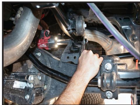
**4.** The pocket on the differential requires trimming for the billet link. Using a die grinder, grind the radius on the pocket gusset as shown. [FIGURE 3 & 4]
