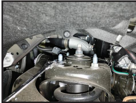
**21.** Lower the control arm and remove the coilover assembly. [FIGURE 20]
