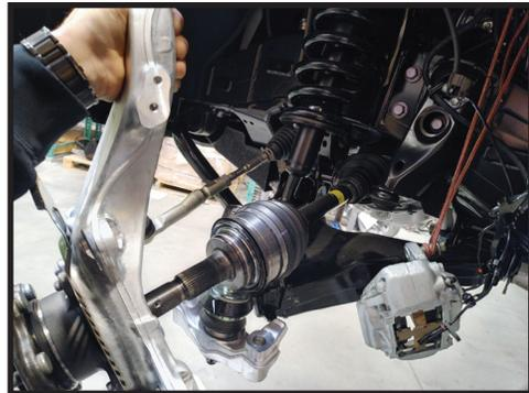
**17.** Use a rope or strap to support the cv/axle assembly out of the way. [FIGURE 17]
