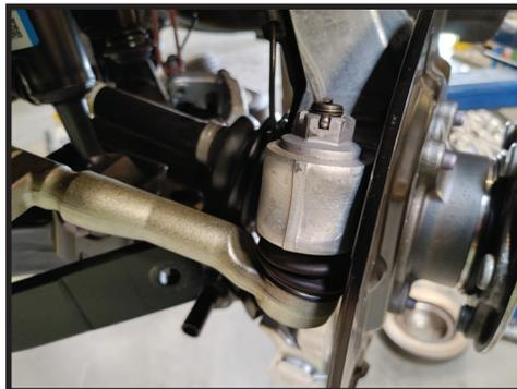
**7.** Use a ball joint separator or a hammer to loosen the tie rod stud taper from the spindle. [FIGURE 6]
