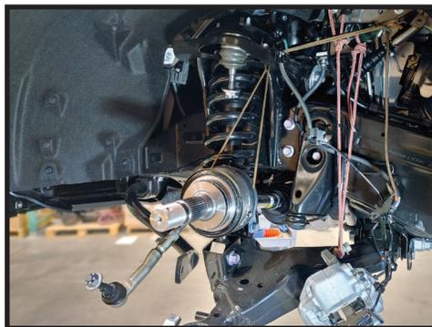
**18.** Support lower control arm and loosen the pivot bolts at the frame using a 24mm.
