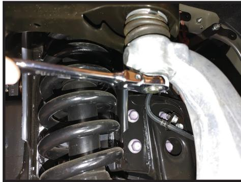
**15.** Use a balljoint separator or a hammer to loosen the balljoint taper from the spindle. Once loose, remove the nut and support the spindle so it does not fall free. [FIGURE 14]
