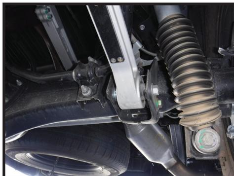
**7.** With the shocks installed. Reinstall the wheels and tires, lower to the ground and torque the lug nuts to factory spec.
