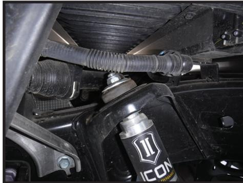
**6.** Install the lower eyelet of the Icon shock onto the axle stud. A deadblow hammer can be used to get the lower eyelet on the stud completely. Use the factory bolt and torque to factory specs. [FIGURE 4]
