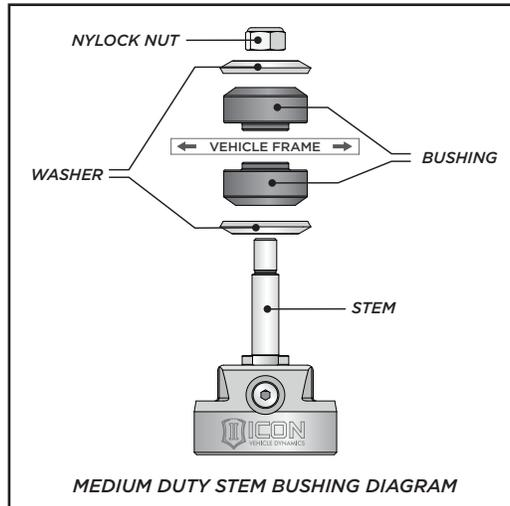
The bushings should center themselves into the factory mount. Thread on the supplied nylock nut until 2-3 threads are showing. [FIGURE 3]
