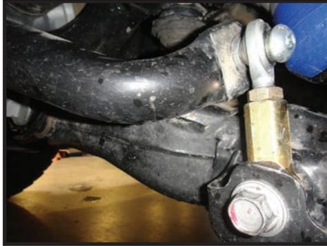
**26.** Remove the factory pinch clamps on the outer end of the tie rod boots on both the driver and passenger side. Slide the tie rod boots approximately 1” inward and fasten using the supplied (605937) pinch clamps. Cycle the steering to make sure that the boots do not contact the shocks at full lock. Failure to check steering clearances may result in steering and/or shock damage. [FIGURE 13]
