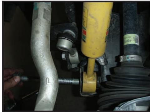
**10.** Support the lower control arm with a jack and remove the bolt holding the shock eye to the lower control arm. Note orientation, this bolt will be reused. [FIGURE 6]
