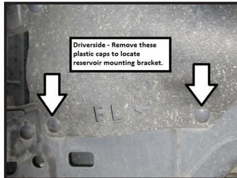
**21.** Mount the reservoir bracket with the front bolt only. Place the supplied adel clamp on the reservoir hose as shown. The rear bolt goes through the adel clamp, and reservoir bracket. This requires you to hold the reservoir in position while putting the bolt in the bracket. [FIGURE 10 & 11]
