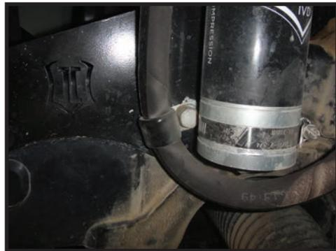
**22.** With the adel clamp in place, and the reservoir positioned on the reservoir bracket, mount the reservoir to the bracket using the supplied hose clamps and a 5/16".
