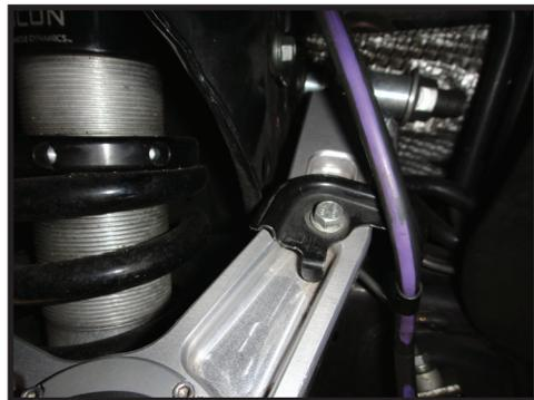
**10.** ICON billet upper control arms utilize heim joints at each pivot to allow alignment using the adjusters on the upper control arms as well as cam adjusters on the lower control arms. The heims can be extended or contracted by turning the collar. Make sure that the slit in the collar lines up with the slit in the housing and then tighten the pinch bolts in an opposing pattern at least 3 times. [Torque to 35 ft-lbs]
