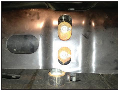
NOTE: If vehicle has a side-lean, install the 10mm spacer supplied in kit. In our experience, the driver side is most often the low side.
