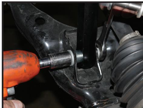
**11.** If replacing the upper control arms, refer to appropriate UCA instructions now. Mount the upper control arm to the knuckle and tighten the taper nut. [Torque to factory spec]
