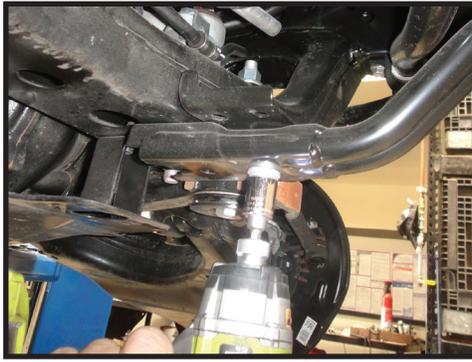
**4.** Disconnect the outer tie rod end on both sides. Remove the cotter pin and loosen the nut until it is flush with the end of the threads. Strike the end of the steering knuckle arm with a large hammer to dislodge the taper. Remove the nut and swing the tie rod out of the way.
