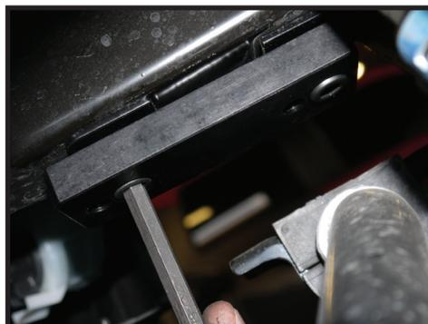
**15.** Install the skid plate braces with the supplied skid plate washers (605432) between the frame and skid plate on all six mounting locations. Use (2) washers per bolt with (3) washers on the bolts towards the front of the truck. Use the supplied (605853) hardware for the middle bolts that go into the protruding bung and the factory hardware for the remaining mounting locations and tighten with a 14mm socket/wrench. [Torque to factory spec] [FIGURE 6]
