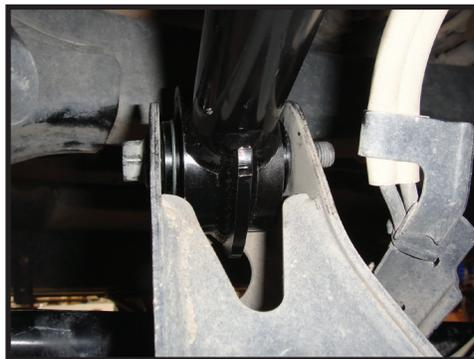
5. The pinion angle can be adjusted as desired once both links are installed. Do not adjust longer than 2.0". [FIGURE 2]
