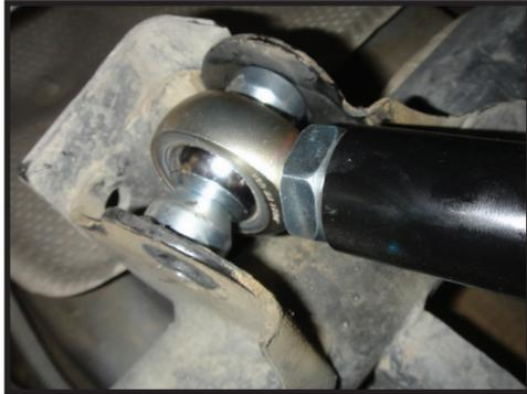
7. Tighten jam nut using an 1.25" open end wrench. [Torque to 120 ft-lbs] Make sure the rod end is vertical as it is tightened.
