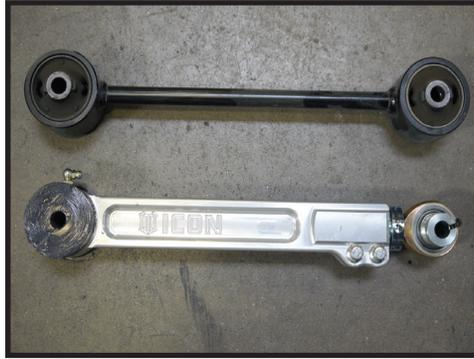
**5.** Install the link. The rod end mounts to the axle and the bushing mounts to the frame. Slide the bolt through the frame end first but do not tighten, next insert the bolt through the axle end.
