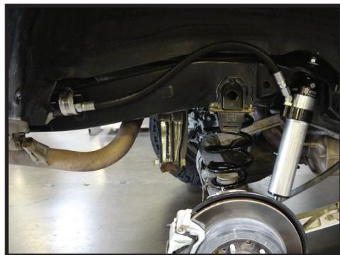
**14.** Install the supplied (605934) adel clamp at the center of the remote reservoir hose in the fender well. Use a 3/8" socket to drive the #14 self drill/tap screw (605033) and secure adel clamp to the pinch weld above the frame in the wheel well. [FIGURE 3]
