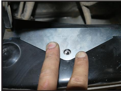
**10.** Using the hole in the bracket as a guide, center punch and drill to 21/64".
