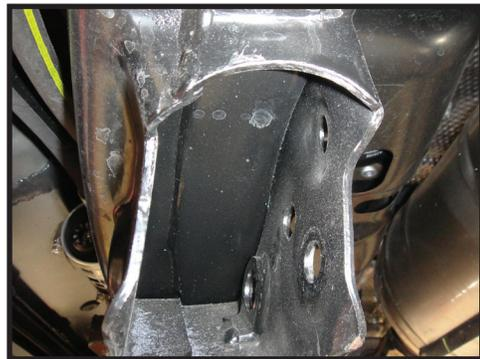
7. Trim as shown. Paint any exposed metal to prevent corrosion. [FIGURE 5]
