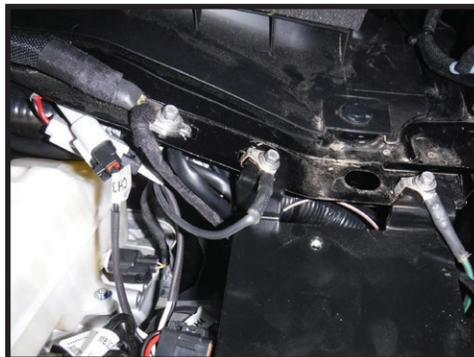
**8.** Tighten the bolt behind the fuse box using a 13MM. [FIGURE 8]
