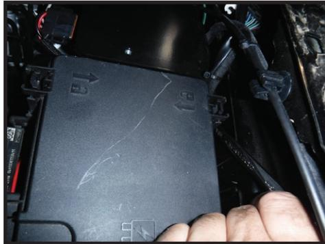
**5.** Connect the IIC mount to the firewall.
