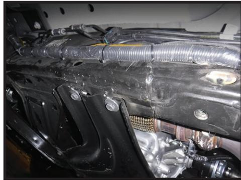
**18.** Connect to the rear driver shock. Be sure to leave enough wire to connect and disconnect from the shock. [FIGURE 16]
