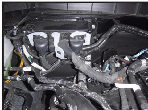
**22.** Route the 10-FT wire down the front of the fender well and plug into shock. Wrap up excess wire and zip-tie in place. Be sure to leave enough wire to connect and disconnect from the shock. [FIGURE 18 & 19]
