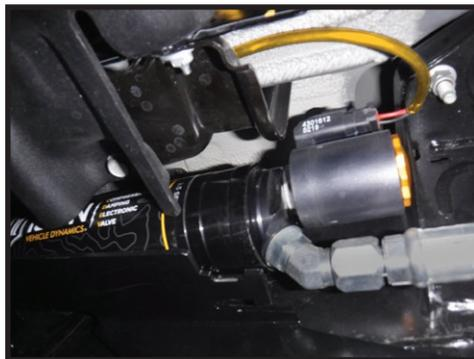
**19.** Connect the 10-FT wire to the Channel-3 plug. Mark the connectors on both sides of the wire PF (Passenger Front). Run it across the firewall and down into the passenger side fender well.
