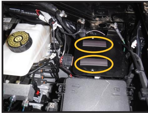
**10.** Connect the IIC (PN 255600) to the mount using the supplied 1/4" hardware and a 7/16". [FIGURE 10]
