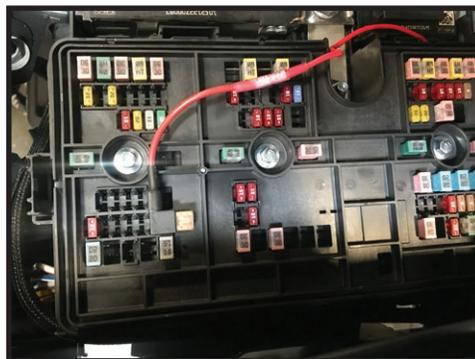
**26.** Route the ACC (Accessory) wire into the fuse box and trim to length.
