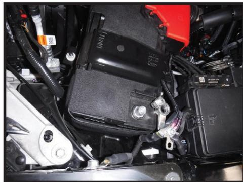
2. V6 MODELS: Disconnect the 2 ground wires from the firewall using an 8MM. [FIGURE 3 & 4]
