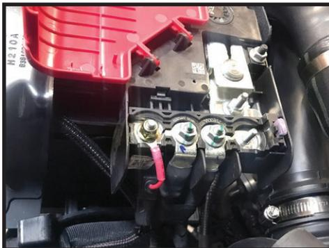
**31.** Trim wire loom as necessary and zip-tie accordingly. [FIGURE 28]
