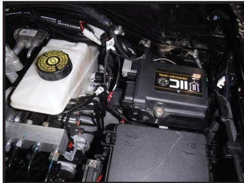
**11.** Connect the grey block off plug (PN 255601) to the grey port of the IIC. Connect the main wiring harness (PN 255602) to the black plug on the IIC. [FIGURE 11]
