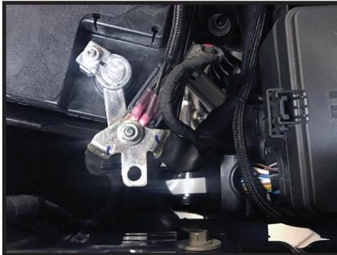
**30.** With the red PWR (Power) wire, route it to the positive battery terminal and cut to desired length. Use the supplied butt connector (PN 605750) to connect the fuse holder (PN 255065-10) to the red PWR (Power) wire. Crimp the terminal connector (PN 605751) to the inline fuse and connect to the positive battery terminal. Use a heat gun to activate heat shrink. [FIGURE 27]
