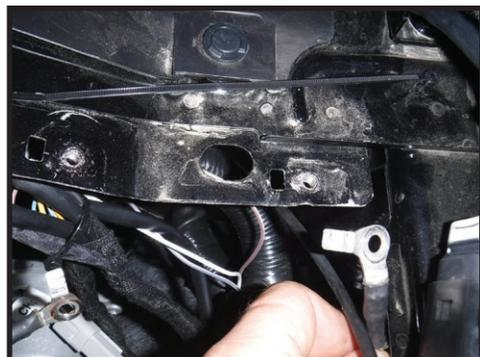
**3.** Loosen the bolt behind the fuse box several turns using a 13MM wrench. [FIGURE 5]
