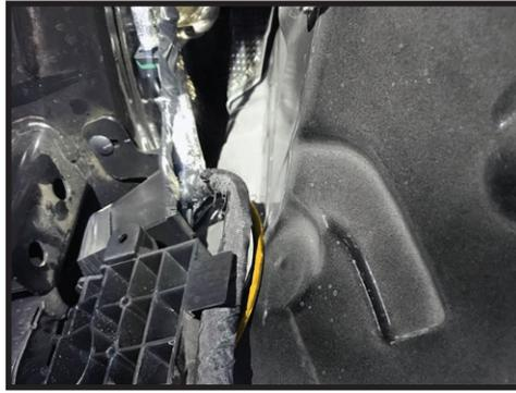
**17.** Route the 14-FT wire down the outside of the driver side frame rail following the wire harness. Wrap up any excess wire and zip-tie to harness along frame rail. [FIGURE 14 & 15]
