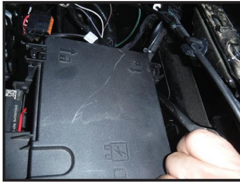
**4.** Slide the open slot of the IIC mount under the head of the bolt. [FIGURE 6]
