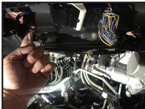
**16.** Route the 14-FT wire to the top of the driver fender and follow the wire harness down the back of the fender. [FIGURE 13]
