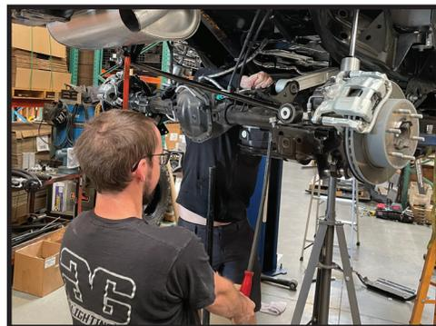
**20.** In order to access the driver side upper link pivot bolt it is necessary to disconnect the exhaust pipe from the hanger at the rear crossmember. Begin by applying WD-40 or other spray lubricant to the rubber isolator [FIGURE 20]. Then firmly grasp the isolator and push it off of the mount [FIGURE 21]. It may require some perseverance to get the rubber isolator past the nub on the metal hanger rod.
