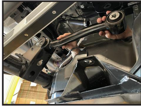
**18.** Insert the bushing end of the passenger side 21-UP BRONCO TUBULAR UPPER REAR LINK into the upper link mount on the vehicle's frame. Reinstall the OE pivot bolt and nut. [FIGURE 17]
