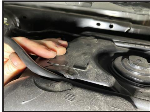
**14.** Carefully lower the fuel tank, taking care to keep it steady and secure on the jack stands as it is lowered. Lower the tank enough to allow access to the lower link bracket on the inboard side of the passenger side frame rail.
