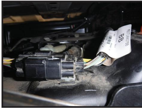
**13.** Near the top-front of the tank, use a body clip removal tool to pull the wiring harness retainer from the retaining hole in the tank (4-Door Bronco only) [FIGURE 10]. Dislodge the fuel line from the groove in the top of the tank. [FIGURE 11]
