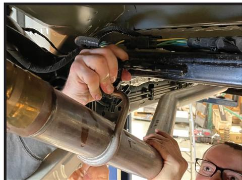
**21.** Continue with installation of the driver side upper link by repeating the previous instructions for the passenger side. When finished, reconnect the exhaust pipe by pushing the rubber isolator back onto the metal hanger rod.
