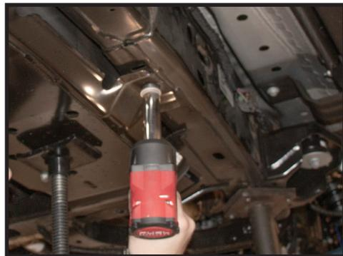
**10.** Slowly lower the fuel tank down a few inches, taking care to keep the tank as level as possible, until you can see and reach the fuel return line on the top of the tank. The line will be located along the side of the frame rail above the tank. The connector will have a white retaining clip on it. [FIGURE 7]
