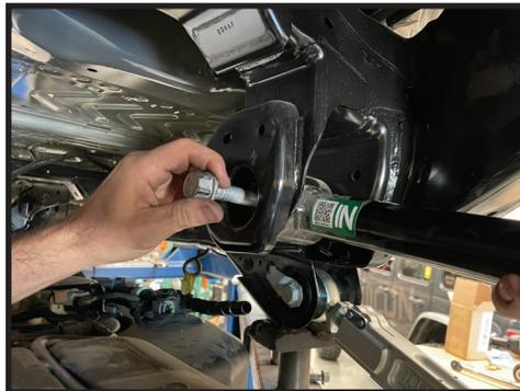
**16.** Note the sheet metal cover that covers the head of the upper link pivot bolt at the axle housing end of the arm [FIGURE 13]. Use a T25 Torx bit and ratchet to remove the two screws and the bolt cover [FIGURE 14]. The cover will not be re-used.
