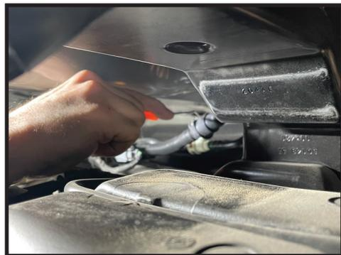
**12.** Disconnect the wiring harness from the top of the fuel tank. [FIGURE 9]
