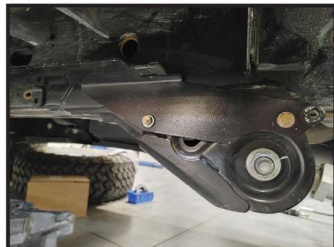
**9.** On the reservoir mount, mark the front hole and drill the frame to 7/32 then use the 1/4" self-tapping bolt to secure the front of the mount to the frame. [FIGURE 8 & 9]
