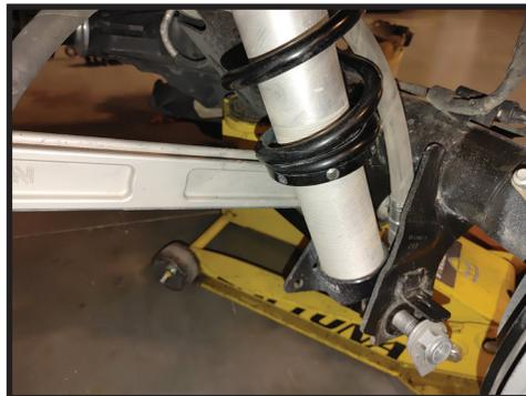
**12.** Route the hose along the lower control arm and place on top of the reservoir mount, using the supplied stainless steel hose clamps to loosely secure it. Then secure the hose to the lower link with the clamps provided with the billet links, or the clamps purchased for the tube links. If non ICON or factory links are installed, cable ties are the next option. [FIGURE 12 & 13]
