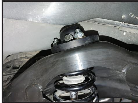
**11.** Install lower shock eyelet with 257194 spacers into the factory mount and torque the bolt to factory spec. (Apply a small amount of anti-seize to the spacers before installing them into the rod end. [FIGURE 11]
