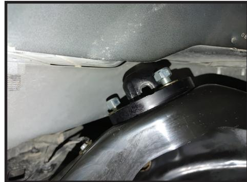
8. Install the reservoir mount to the frame above the lower link pivot. Use the supplied 1/4" nut plate and 1/4" bolts and washers. Grind any high spots in the factory weld to allow the reservoir mount to sit flush against the frame. [FIGURE 6 & 7]
