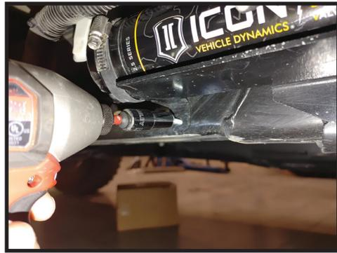
**10.** Install the Icon coilover into the upper mount with the 257172 spacers and 605334 1/2-13 12pt bolt. (Apply a small amount of anti-seize to the spacers and bolt.) Torque to 90 ft-lbs with a 1/2" 12pt socket. [FIGURE 10]
