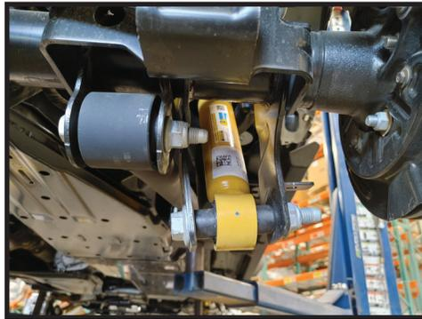
7. Install the upper mount and stud plate as shown, the stud plate installs from under the frame mount, and the upper mount installed on top of the frame with the 2 studs/nuts accessible from the wheel well and the 7/16" bolt towards the inside. (Driver side shown) Torque the 7/16 bolt to 65 ft-lbs. Torque the 12mm nuts to 65 ft-lbs. [FIGURE 5 & 6]
