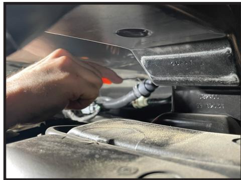
**10.** Disconnect the wiring harness from the top of the fuel tank. [FIGURE 9]
