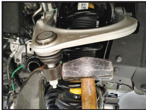
**6.** Support the spindle so the CV joints do not overextend and remove the balljoint nut.
