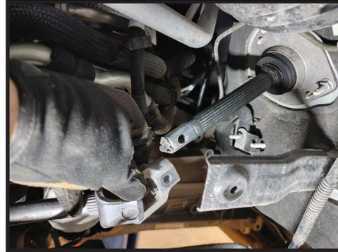
**5.** Remove balljoint from the spindle using an 18mm, leave the nut on loosely. To free the taper from the spindle, a hammer or balljoint separator can be used. [FIGURE 4]
