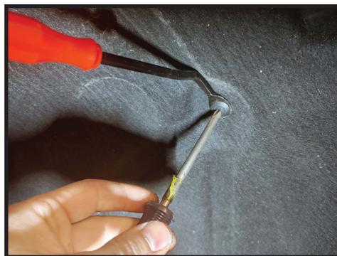
**3.** On Driver side only, disconnect the steering shaft coupler. Remove the 10mm bolt and push the black grooved shaft into the body. Before removal, make sure the steering wheel is straight. Do not turn steering while disconnected.
