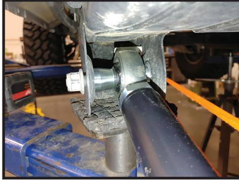
**18.** Insert the bushing end of the ICON link arm into the lower link mounts on the axle housing. The link will be offset in the axle housing, with the wide spacer towards the center of the vehicle. It may be necessary to carefully tap the link into place using a soft dead-blow mallet to avoid marring the anodized finish of the arm. Re-install the modified pivot bolt (with the shortened retainer tab) and tap it into place. [FIGURE 16]
