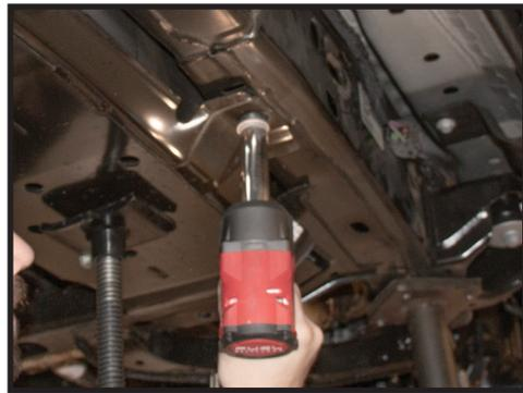
**9.** Slowly lower the fuel tank down a few inches, taking care to keep the tank as level as possible, until you can see and reach the fuel return line on the top of the tank. The line will be located along the side of the frame rail above the tank. The connector will have a white retaining clip on it [FIGURE 7]. Remove the retaining clip and disconnect the fuel line [FIGURE 8]. A small pick may be used to carefully pull the retaining clip.
